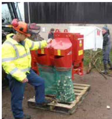
Welmac branch logger at Elm Farm.
