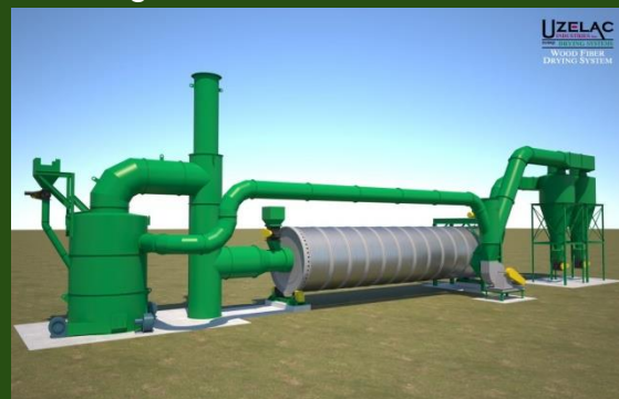
Figure 2. Rotary drum wood chip dryer ( http://www.uzelacind.com )
